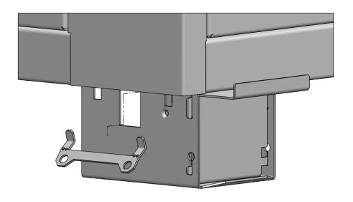
2. Rotate and drop out locking tabs.
