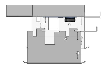
3. Slide each foot towards the center of the rack. 4. Rack can now be lifted, and each foot should drop out.
