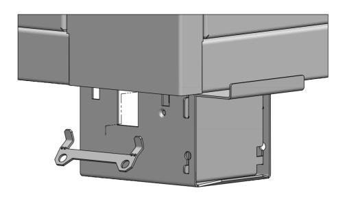
2. Rotate and drop out locking tabs.
