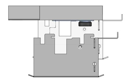
3. Slide each foot towards the center of the rack. 4. Rack can now be lifted, and each foot should drop out.
