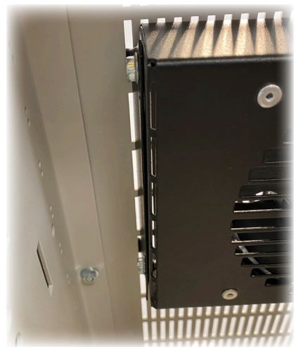
secure screws to complete fan tray installation
