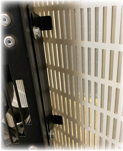
align the bracket with the venting
