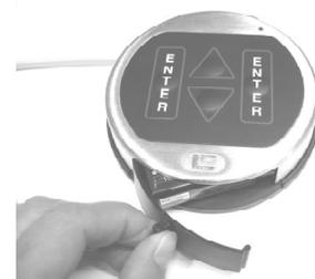
**ONLY USE ALKALINE BATTERIES**- other varieties will cause irreparable damage to the lock mechanism and could lead to failure and lockout
