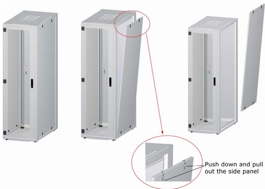
**Replacement:** The side panel has a “top” and a “bottom”. The top is identified by semi circular notches in the vertical flange (edge) near the top. Normally, the orientation of a Side Panel will maintained when it is removed and replaced, as it is convenient to store Side Panels vertically.
